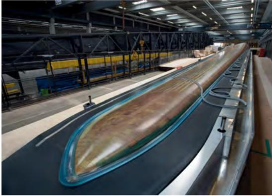
Figure 3: Wind turbine blade right after molding.
