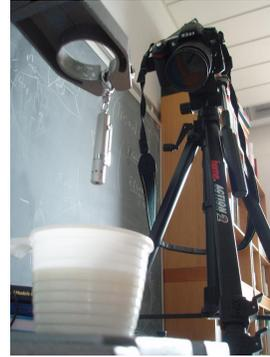
**Fig. 4.2** A simple experimental setup where we can take a picture of a laser pointer shining light into a cup of milk.
