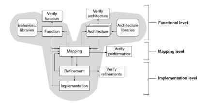
Figure 1.1: Embedded system design methodology. Source: [35]
