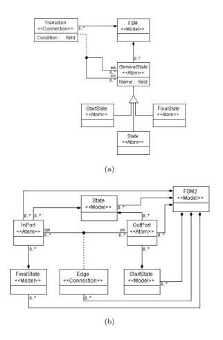
Figure 4.6: Two different meta-models of finite state machine.
