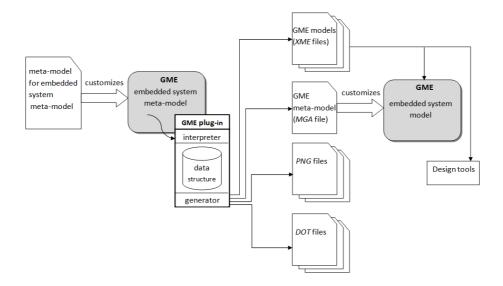
Figure 1.2: Process of model generation using GME and the Model Generator plug-in.
