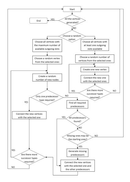
Figure 5.1: The flowchart representing the synthetic model generation algorithm.
