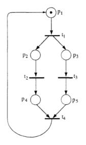
Figure 2.2: Example of a simple Petri net. Source: [36]
