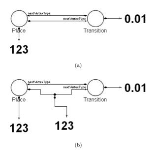
Figure 6.7: Meta-models of a marked Petri net with multiple edges represented as: (a) parallel edges, (b) as a parameter associated with a connection type.
