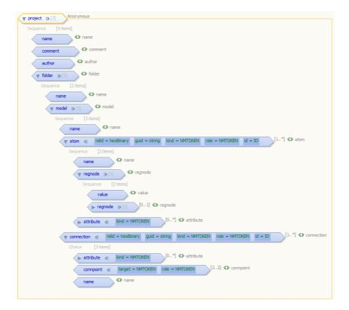
Figure A.2: XML Schema of a GME model in XML format
