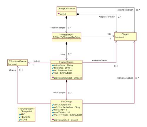
Figure 4.4: A class diagram specified using EMF. Source: [2]
