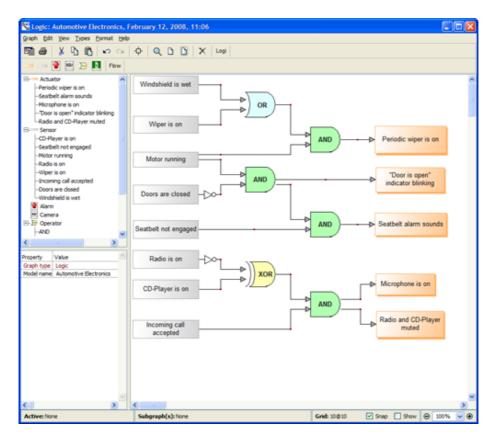
Figure 4.3: MetaEdit+ modeling environment for arithmetic logic. Source: [1]
