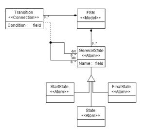
Figure 4.1: A finite-state machine meta-model
