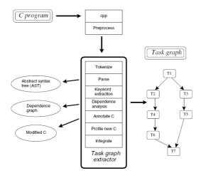
Figure 3.3: Process of a task graph extraction from C code files. Source: [31]
