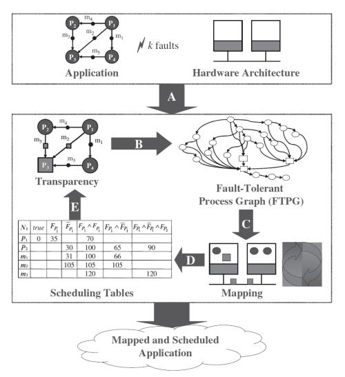
Fig. 1. Overall synthesis flow.
