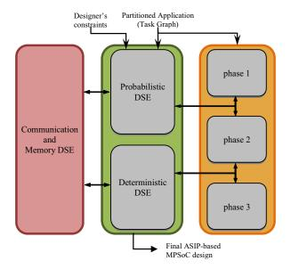
Figure 3 System Level DSE
