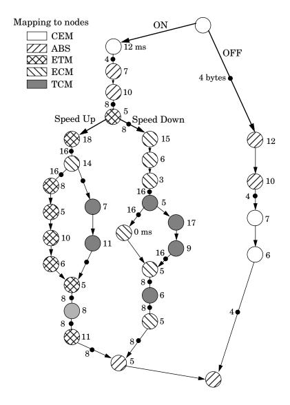
Figure 6.2: Cruise Controller Model
