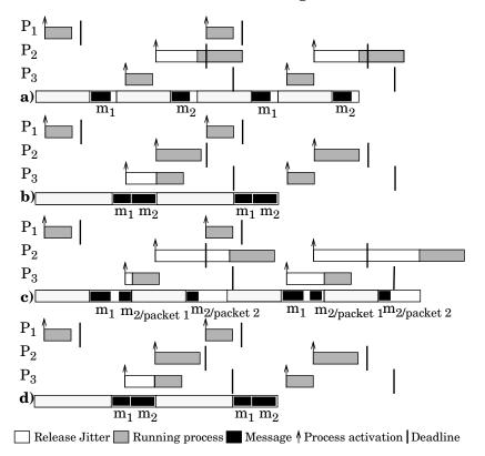
Figure 5.3: Optimizing the MEDL for DM and DP
