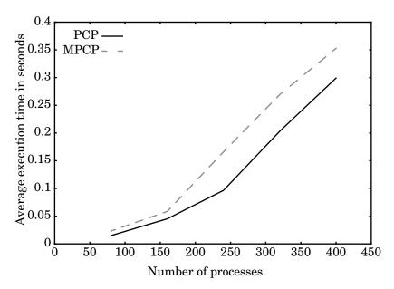
Figure 4.10: Average Exec. Times of PCP and MPCP
