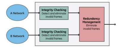
Figure 2.21: "Receive Processing of Ethernet Frames." Figure. [Pla05], 13p.
