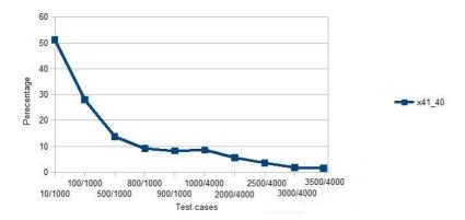
Figure 5.5: Percentile difference between the 1000, 1500, 2000, 2500, 3000, 3500 with respect to 4000 Simulation runs
