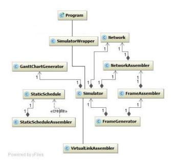
Figure 4.2: Simulator. UML diagram.
