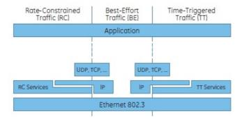
Figure 2.11: "Relation of TTEthernet to existing communication standards." Figure. [TSPS12], 10p.
