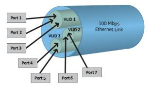
Figure 2.5: "Three Virtual Links Carried by a Physical Link." Figure. [Pla05], 14p.
