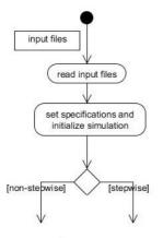
Figure 4.9: Simulation initialization. Activity diagram.
