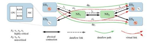
Figure 2.10: "TTEthernet cluster example." Figure. [TSPS12], 3p.
