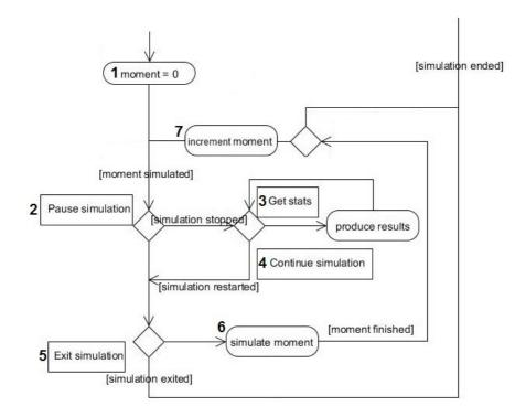
Figure 4.8: Stepwise simulation. Activity diagram.
