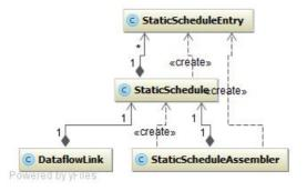
Figure 4.4: Dataflow links use StaticSchedule. UML diagram.
