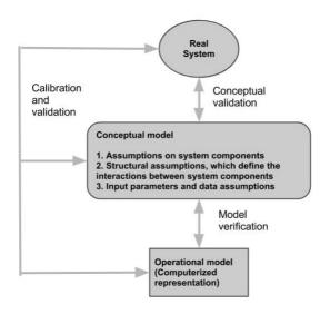
Figure 3.3: "Construction of a model". Figure. [BCNN00]
