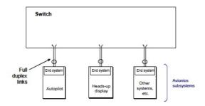
Figure 2.1: "Full-Duplex, Switched Ethernet Example" Figure. [Eng05], 12p.
