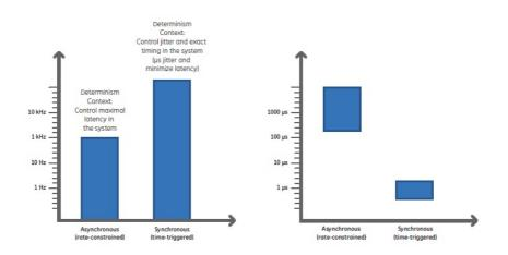
Figure 2.2: "Determinism context in Ethernet networks depends of the application (max. sampling rate) and the approach to system design asynchronous (coordination and synchronization among functions is conducted at higher layers) or synchronous (control of timing and synchronization at network level)." Figure. [Pla09a], 4p.
