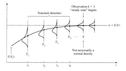
Figure 3.5: "Transient and steady-state density functions". Figure. [LK99]
