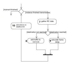
Figure 4.14: A frame instance finished transmitting. Activity-oriented implementation. Activity diagram.
