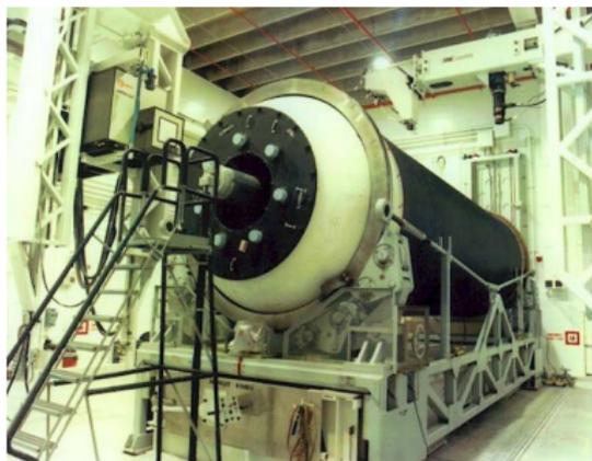
Exterior CT is used for nondestructive evaluation (NDE) of rockets because industrial X-ray CT scanners can't penetrate the thick central part of the rocket, but they can penetrate the outside annulus. Often scientists are interested in cracks, etc., in the rocket shell, anyway.
