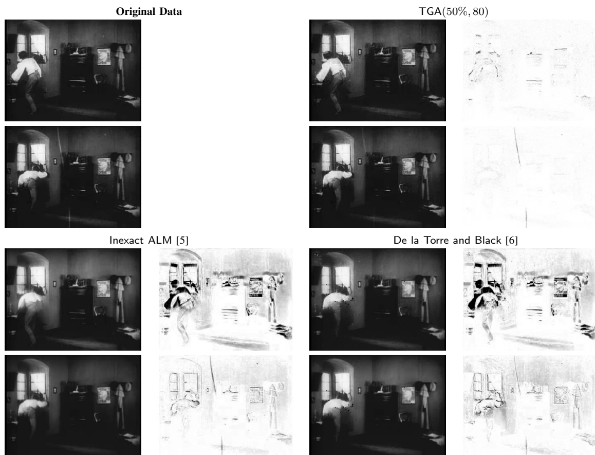
Fig. 5. Two representative frames from the 1922 film Nosferatu as well as their restoration using TGA and the algorithms from [5], [6]. TGA removes many outliers and generally improves the visual quality of the film, while Inexact ALM oversmooths the results and De la Torre and Black oversmooth and introduce artifacts. This is also seen in the absolute difference between the data and the reconstruction, which is also shown (inverted and multiplied by 2 for contrast purposes). We also refer the reader to the supplementary video.
