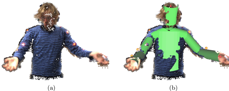
Fig. 2. (a) A segmented stereo image of a human body. (b) A human skeleton estimate projected on the image data.
