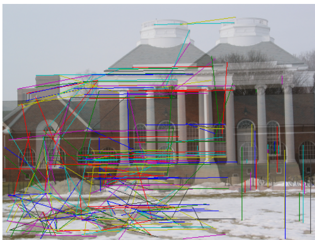
Figure 1.10: Putative matching points connected by lines. Points are from Fig. 1.9, and include those that gave the highest cross-correlation match. Outliers (non-horizontal lines) and inliers (horizontal or near-horizontal lines) can be easily distinguished.
