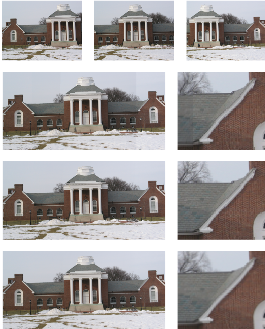
Figure 1.6: Comparison of stitching variants. Row 1 : The original three images to be stitched. Row 2 : Rounding used for interpolation, and averaging for the overlapping parts. Row 3 : Rounding used for interpolation, and hat-function weights for the overlapping parts. Row 4 : Bilinear interpolation used for interpolation, and hat-function weights for the overlapping parts. Right : Detail of images. The computation time for the three methods: 13.8 seconds, 14 seconds, and 73 seconds on the same machine.
