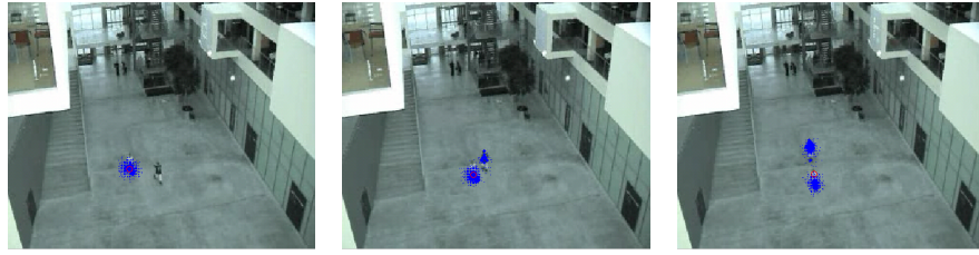
Figure 3.12: Three equally spaced frames illustrating the split of the particle set when tracking a person walking in ITU building. Settings used: number of particles N = 1000 , standard deviation for random propagation \Sigma = 5\mathbf{I} .
