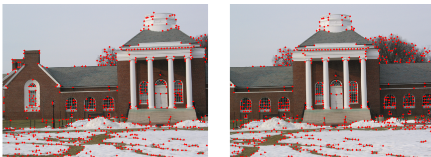
Figure 1.9: Points output from Harris corner detection on two overlapping images.
