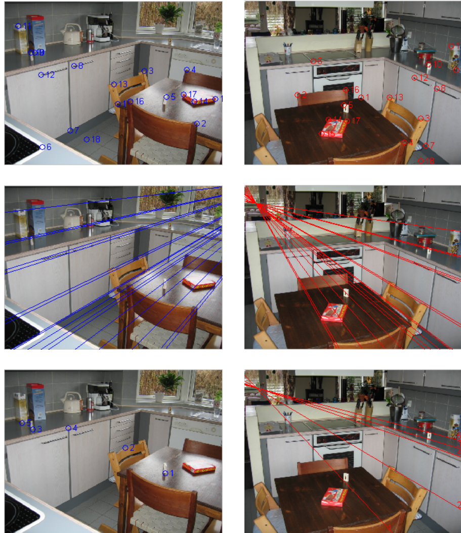
Figure 2.8: Estimation of the fundamental matrix using the 8-point algorithm. Top row : Point correspondences used for estimation of F . Middle row : Epipolar lines determined by the corresponding points. The epipoles (locations where epipolar lines meet) reveal camera locations: the epipole in the left image is where the camera was when the right image was captured, and vice versa (the left epipole is outside the boundary of the image). Bottom row : Testing points and the corresponding epipolar lines.
