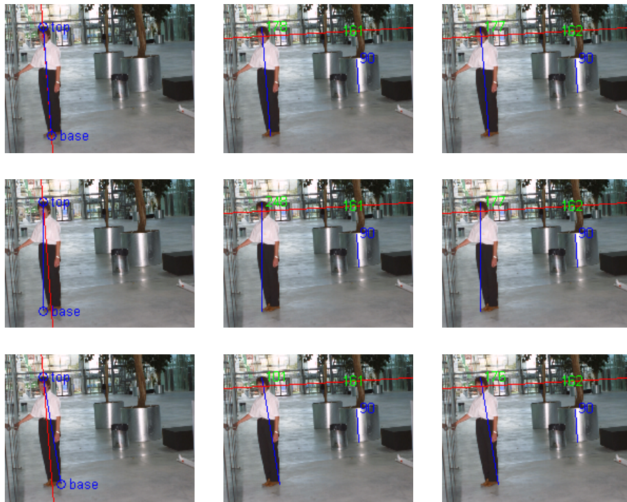
Figure 2.6: Comparison of algebraic (middle column) and geometric (right column) method. Top row : Well chosen top and base points. Middle and bottom rows : Poorly chosen top and base points.
