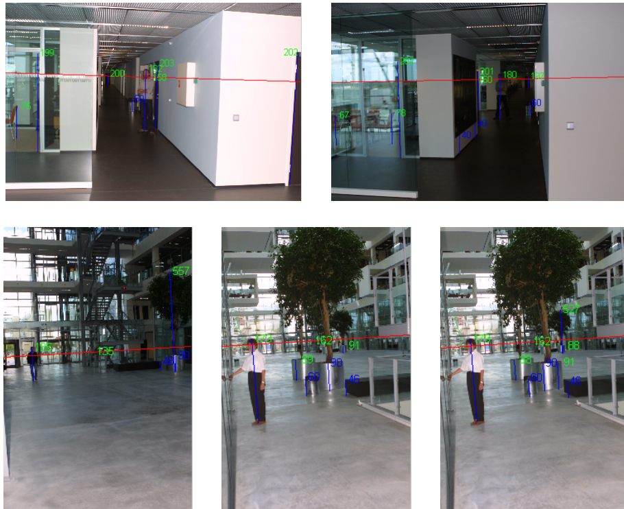
Figure 2.5: SVM results. Top left : Four heights that were calculated from a single reference height. Top-right : Three reference heights used for metric calibration. Bottom row : Further examples of height estimations. Reference heights are shown in blue, calculated heights are shown in green, and the horizon is given in red. The camera height is given in green, and can be found near the middles of the horizon lines.
