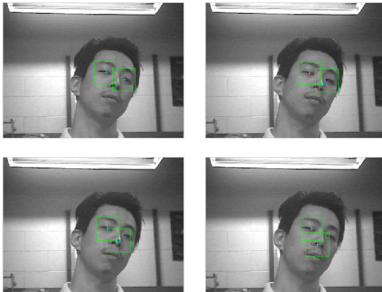
Figure 3.7: An example of unsuccessful tracking, caused by the uncertainty region being too large.
