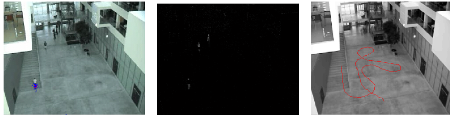
Figure 3.13: Successful track of the person walking. Left : A frame from the tracking sequence with the particles plotted on top. Middle : Corresponding difference image, which was a base for evaluating the particle weight. Right : Final path; should be compared with the figures in Section 1.4.
