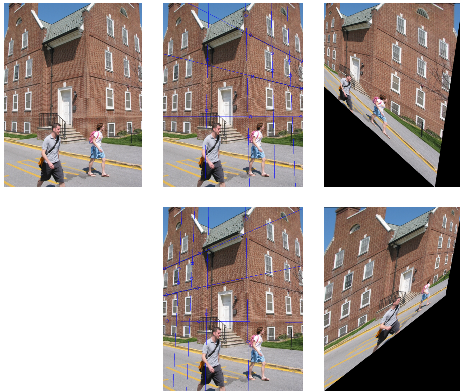
Figure 1.14: Two affine rectifications of a single image. Top-left : The original image. Center column : The selected planes. Right column : Affine rectification of the left and right sides of the building in the original image.
