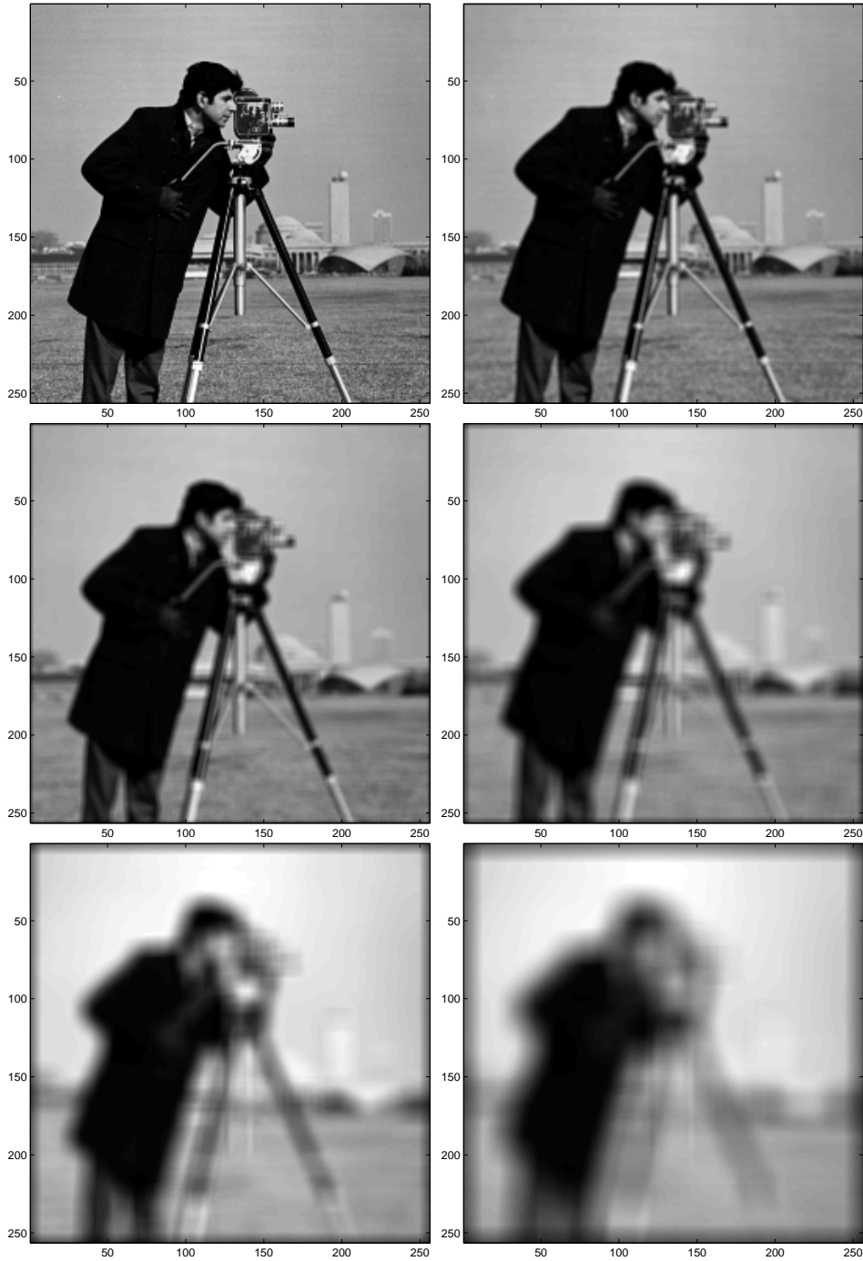
Figure 2: Left to right, top to bottom: original image, of size 256 \times 256 pixels, and images smoothed using averaging_filter function with the filter sizes k = 3, 5, 9, 1, 25 pixels.
