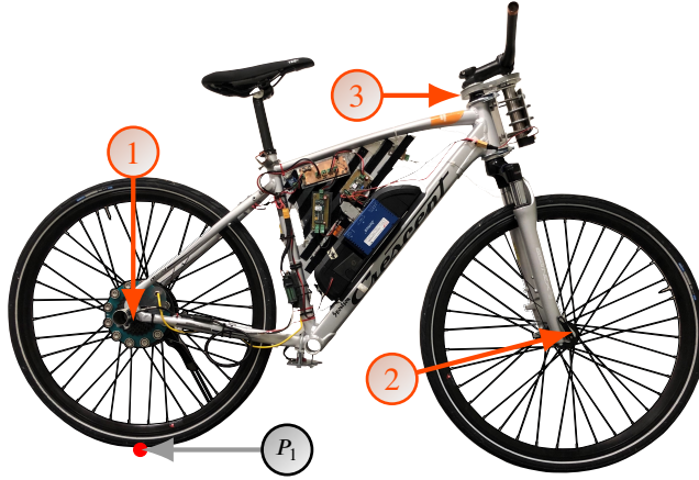
Figure 9.2: Instrumented bicycle with three revolute joints highlighted as 1, 2 and 3. P_1 represents the contact point between the rear wheel and the ground.
