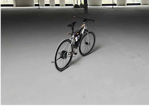
Figure 5.4: The instrumented bicycle controlled through a unified control framework consisting of FL and DeePO.
