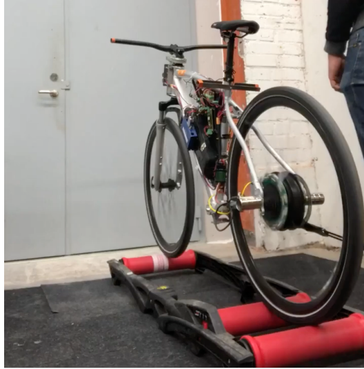
Figure 5.3: Experimental setup in Paper A where an autonomous bicycle is riding on a bicycle roller.
