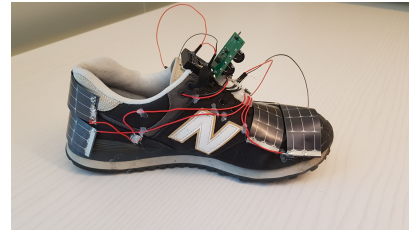
Figure 2: The smart-shoe prototype designed based on a regular shoe
