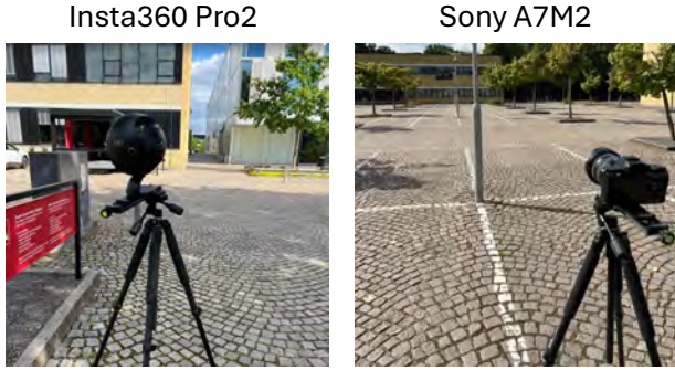
Figure 3. Capture settings. Both the Insta360 Pro2 and Sony A7M2 are mounted on a rail system to enable front-to-back adjustments for precise alignment with the nodal point.
