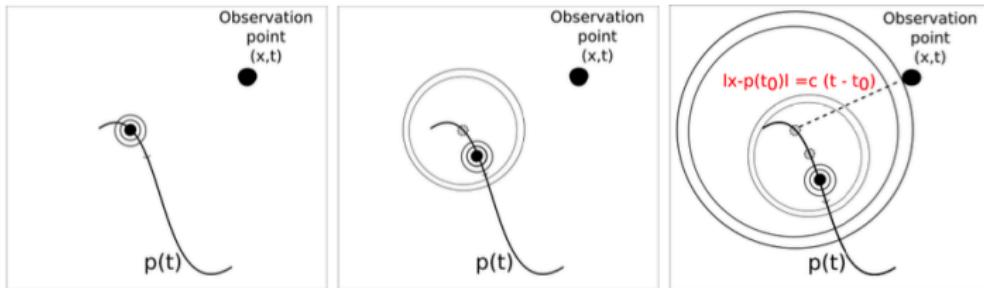
**Figure 2.1:** The emission of a wave from a moving source as time increases from left to right.
