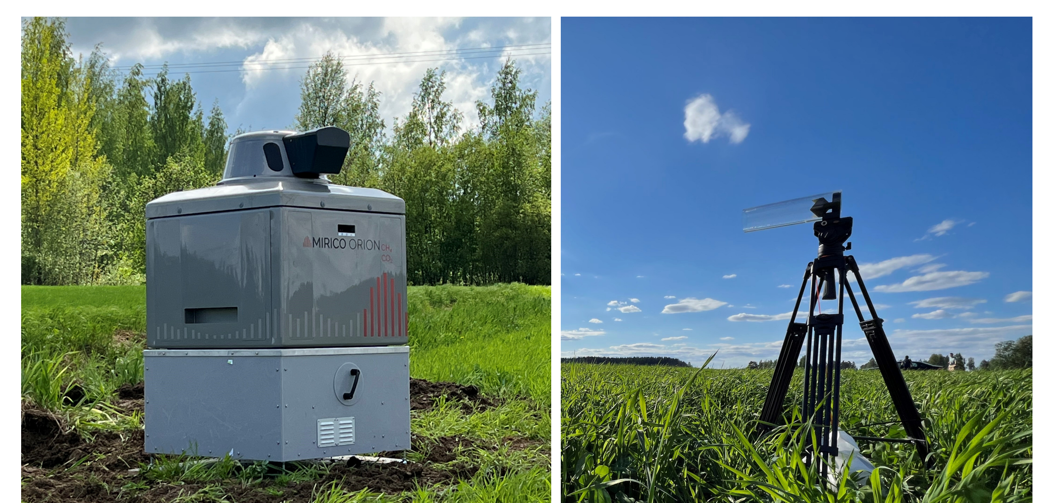
FIGURE 4: MIRICO ORION DUAL GAS (CO 2 , CH 4 ) ANALYZER IN AGRICULTURAL FIELD.
