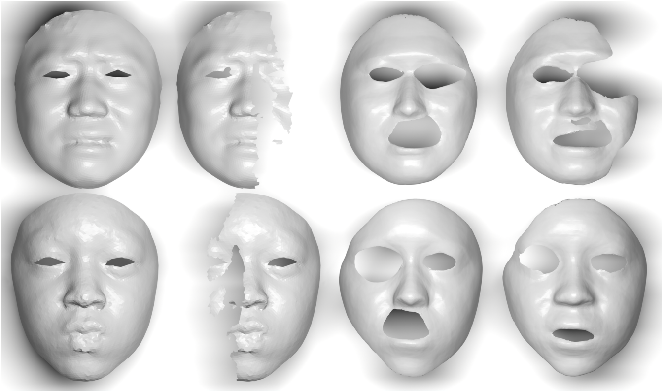
Figure 10: Partial shape reconstruction from the BU-3DFE dataset [YWS*06]. From left to right: ground truth, simulated partial shape, GWN reconstruction, SSDF reconstruction. The simulated partial scans contain 61% and 59% (top and bottom) of the original surface.
